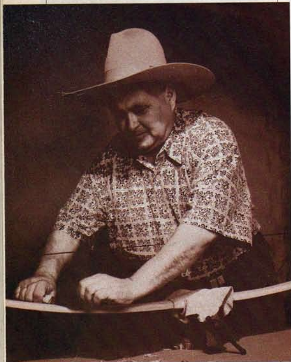
Since both ends of the bow must be equal in strength, Peter A. Roybal administers the final shaping with a draw knife or rasp.
